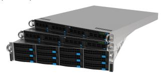
The Capture Cloud Managed Video Recorder (CMVR) stores video and acts as a gateway from your premises to the Capture Cloud Data Center where your video canalso be stored and managed by the Capture Cloud VMS. It provides video storage, video buffering, a secure connection, bandwidth management, and monitoring ofcameras.
