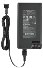
PS-1225UL® 12V DC, 2.5A Power Supply for LEF Series with All Call or TD-H Series (required for the LEF Series if using BG-10C, otherwise use PS-1208UL)
