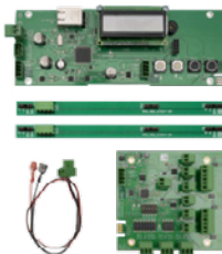
ACS-2DR Two-Door Access Control Starter Kit (includes one door master controller, one AC-2DE expander board, and two AC-STRIPs—included with ACS-2DR-C kit and is sold separately for AC-CA1 enclosure, p. 13)
