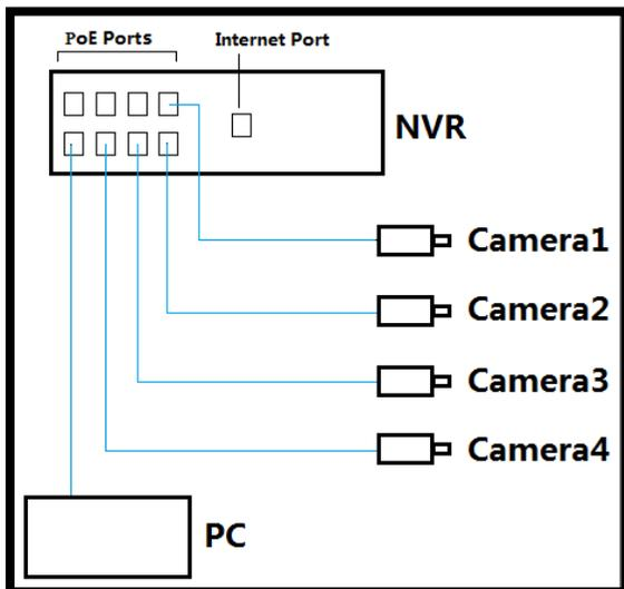
2. Make sure that the cameras' IP addresses and the Internal NIC IPv4 address of the NVR are on the same IP address range. First, check the Internal NIC IPv4 address on the NVR. [Menu > Home > Network](#)
