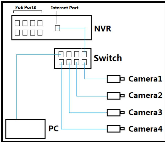
2. Make sure that the cameras and the NVR follows the IP range of the router. Check the IPv4 address of the NVR. [Menu > Home > Network](#)
