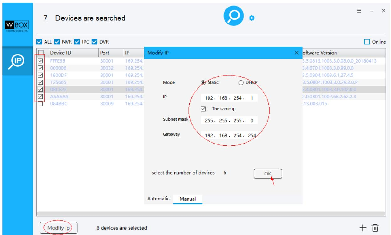
The screenshot shows the IP Search Tool interface. At the top, it says "7 Devices are searched". Below this, there are filters for "ALL", "NVR", "IPC", and "DVR", all of which are checked. A table lists the devices with columns for "Device ID", "Port", "IP", and "software Version". The first six rows are selected, and their IP addresses are 169.254.x.y. A "Modify IP" dialog box is open, showing the following settings:
