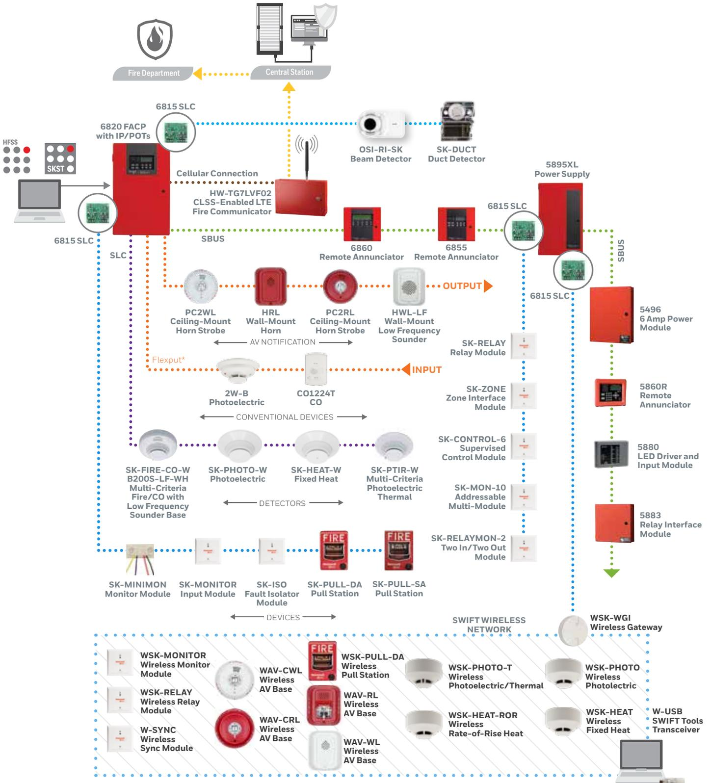
\* Flexput Circuits are input or output circuits that can be programmed for NACs, conventional input circuits, or auxiliary power - constant power, door power, or resettable smoke power. Versatility without the cost of additional modules. Also useful for retrofitting existing systems.
