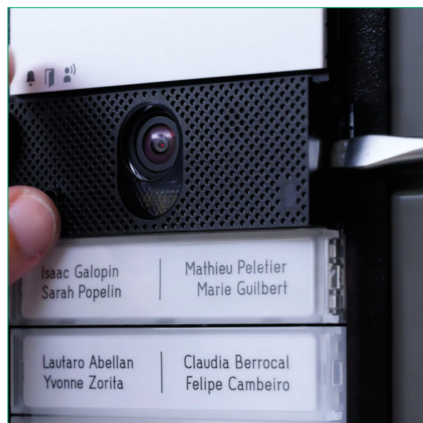
8. REMOVE the front panel to access the various programming modes/settings
