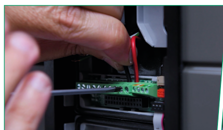
5. POWER the modules and CONNECT the door lock, if any
