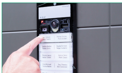
10. PRESS the button to which the address selected in the previous step will be assigned. An acoustic signal sounds to confirm that the address has been correctly assigned. By SELECTING the other buttons in succession, they automatically acquire the call address with the next code
