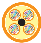
48-fibers (4 tubes of 12-fibers)
