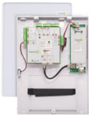
Paxton10 - Single-door controller, PoE
