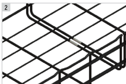
2 Position tray so that the exposed conductive tape are aligned and use SWKs to join tray sections.
