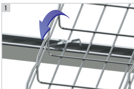
1 Hook one side of the FS41 into channel support.
