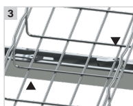
Add an additional FS41 on the opposite side of the channel support for secure installation.
