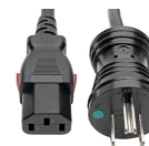
P006-L06-HG10 5-15P to Locking IEC C13, Green Dot, 10A, 125V, 18 AWG, 6 ft., Black
