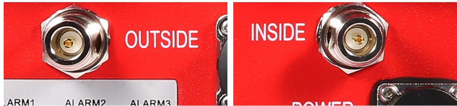
A1 — N-type Female for OUTSIDE cable and antenna
