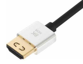
These slim HDMI® cables are designed to handle up to 10K@30Hz resolutions with HDR and boast an impressive 48Gbps bandwidth speed. The Enhanced Audio Return Channel (eARC) supports advanced audio formats such as DTS Master, DTS:X, Dolby TrueHD, Dolby Atmos, and more. Plus, the SecureFit connectors are pull-tested up to 7lbs and provide 45% stronger connections than regular HDMI™ cable ends, ensuring exceptional strength and durability.
