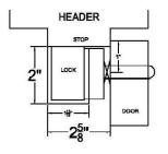
ON FULL WIDTH STOP WITH SURFACE MOUNTED ARMATURE
