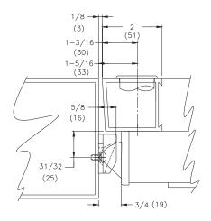
Locate mounting hole on inactive stile.
