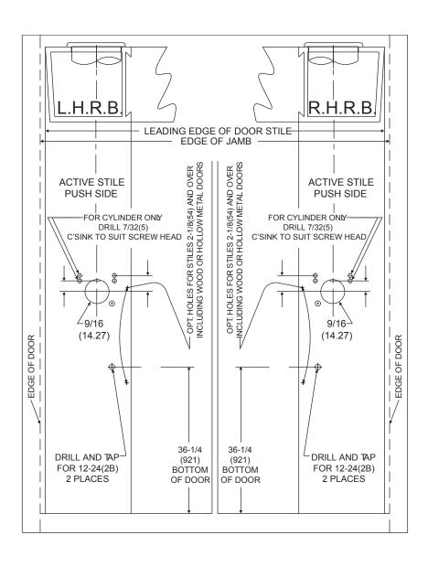
Locate centerline of cylinder on exterior of door and drill if required.
