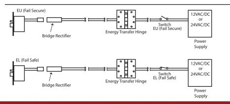
STEP 4: Connect the wires exiting the mortise pocket to the Bridge Rectifier (included).
