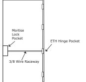
**STEP 2**: Run the wires from the ETH hinge through the 3/8" raceway starting at the ETH hinge & exiting into the mortise pocket.
