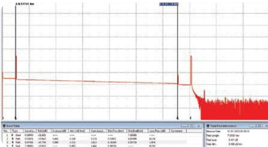
TraceViewer with expanded trace view highlighting the benefit of Launch Cables to examine Near & Far end connectors.
