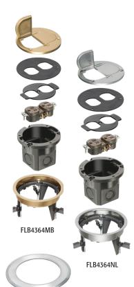
4" round, UL Listed metallic floor box kits with low profile steel bracket for existing floors. Designed for flush-to-floor, neat installations. Quickly install with a SINGLE hole saw. The cover seats into the matching low profile, 0.040" thick plated steel bracket, sitting flush with the floor and reducing trip hazards.
