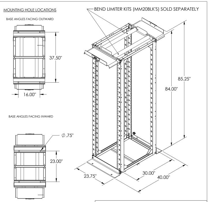
TESTED TO UL2416 WITH A WEIGHT LOAD OF 2000LBS.
