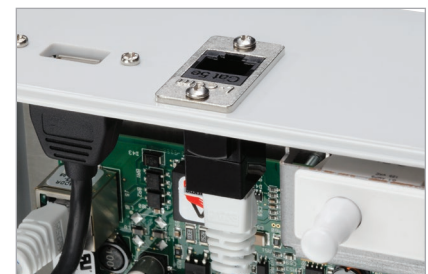
PIM400-1501-LC has RJ-45 and USB external connectors to make installation easy.
