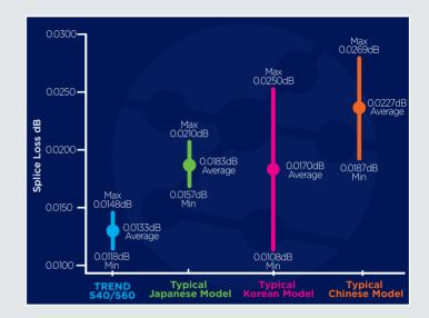
Maximum allowed splice loss for installations that comply with ISO/ EN/TIA standards is 0.30dB. FiberMASTER splice loss exceeds these standards by more than 20x, reducing attenuation in your fiber links and increasing overall system margin. Data from 100 splices measured with laboratory test equipment. Not the loss displayed on the fusion splicer screen.
