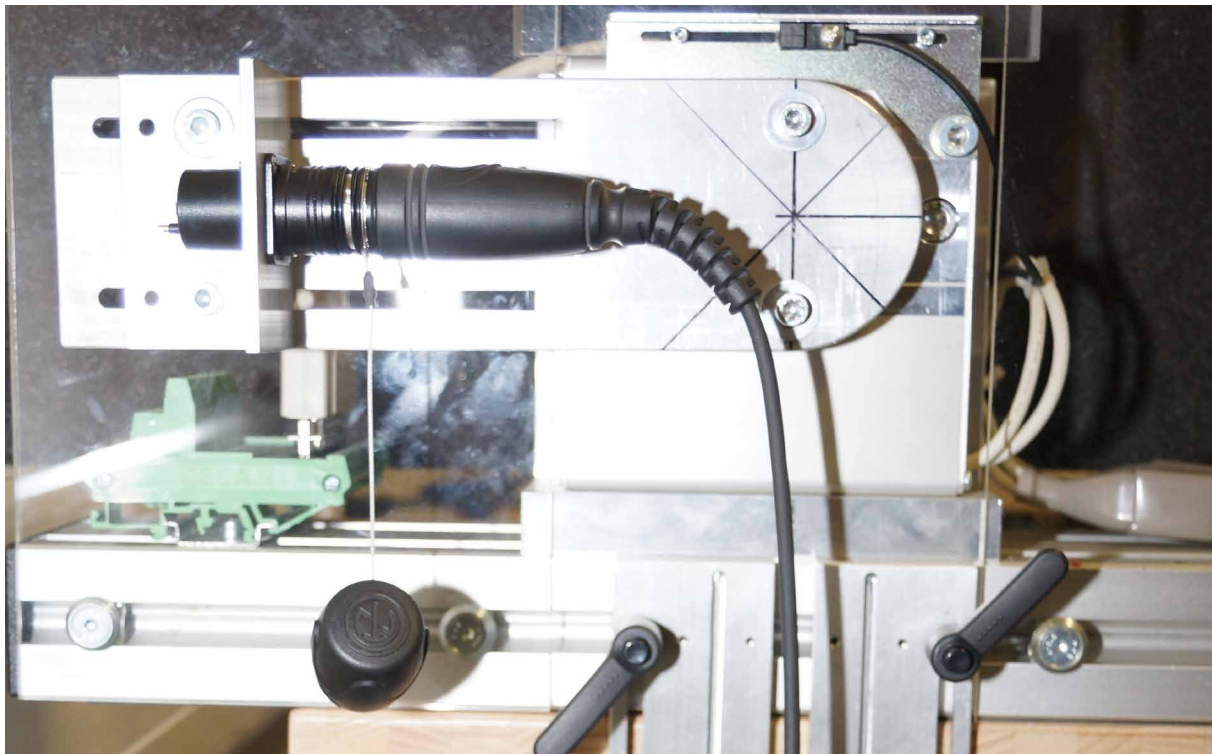
figure 9.b: Test Equipment and Fixture for flexing test
