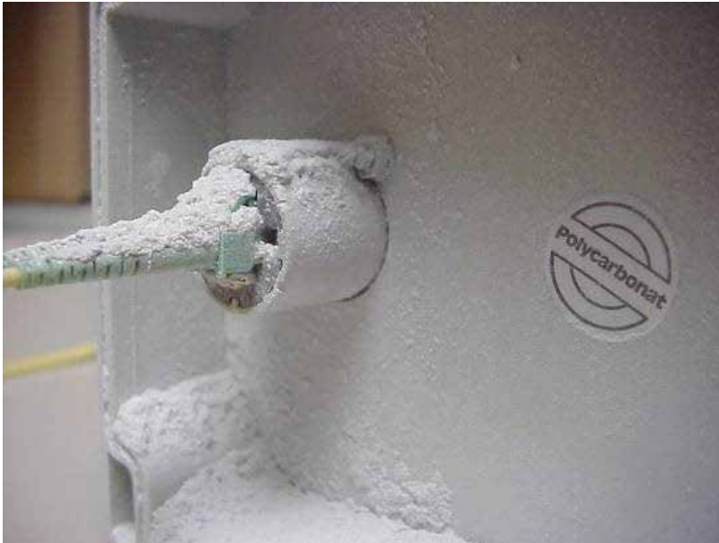
figure 10.b: Dust sediment on the rear side of the receptacle after 60 min.
