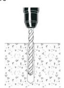
Where a fixture is used, drive the anchor through the fixture into the anchor hole until the head is firmly seated against the fixture. Be sure the anchor is driven to the
