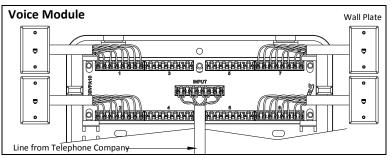
**Step 3a**: Terminate the incoming phone line to the 110 IDC labeled "INPUT". Identify each outlet cable and terminate to 110 IDC labeled "1~8". Note: Line #1= Blue, Line #2=Orange, Line #3=Green, Line #4= Brown.
