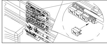
**Optional:** To protect termination wires and debris from entering 110 connectors, termination cap can be use (sold separately).
