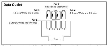
**Note**: It is important to follow T568A wiring because it allows pair 1 and 2 to be used for phone applications, up to 2 lines.
