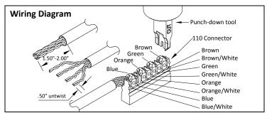
**Step 2**: Terminate the wires by only using a 110 punch-down tool. Be certain to follow the specified T568A color code for 8P8C installations as per TIA-570 residential wiring standards.
