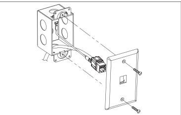
Step 2a: Ground the wire to the metal electrical box by screwing down the fork terminal or follow step 2b.
