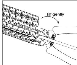
Step 1. Clamp the tool onto the connector. Step 2A. To remove connectors from the Step 2B. To remove connectors from the tool gently and slightly downward.
