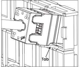
Step 2A. Insert the top row by tilting up 45 Step 2B. Insert the bottom row by tilting down The upper row of the connectors are installed degrees with the tab down.
