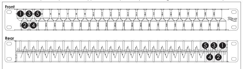
Step 1. Insert connectors into the patch panel in staggered order. For example, start with Port 1, then Port 25, then Port 2, then Port 26, and so on.
