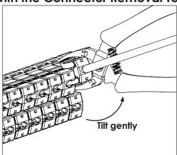
Note: Connector will break if tool is not placed top row, squeeze the tab and tilt the tool bottom row, squeeze the tab and tilt the gently and slightly upward.
