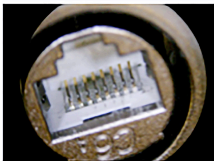
figure 14 – NE8FDX-Y6 after 1000 mating cycles
