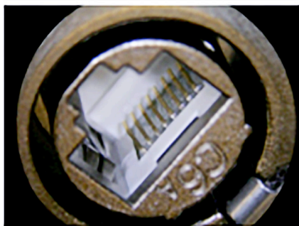
figure 12 – NE8FDX-Y6 before test
