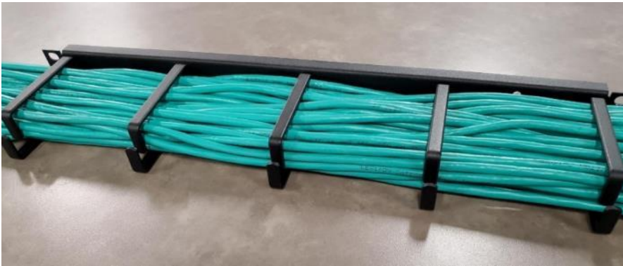
50% Fill Ratio of 6.0mm Patch Cords in 49253-LPM Ring-type Cable Manager (44 Cords). Even though 44 cords “fit” into the rings, this cord density is impractical for most horizontal cord manager applications.
