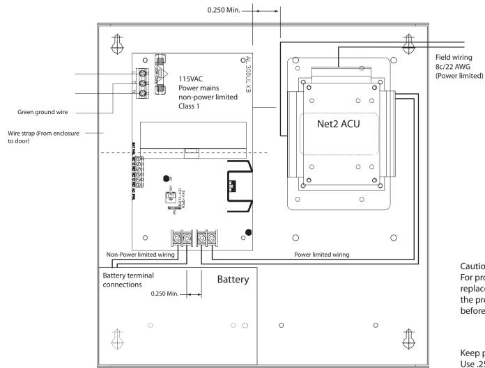
Caution: De-energize unit prior to servicing or ACU installation. For protection against risk of electric shock and fire hazard replace fuse with the same type and rating, 3.5A, 250V. Replace the protective cover on the fuse of the AL300ULXB board, before energizing the unit. Do not expose to rain or moisture.
