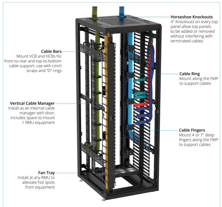
84"H x 29"W x 32"D frame shown, four top cabinet knockouts are part of 29" frames only, not all accessories shown are compatible with smaller cabinets
