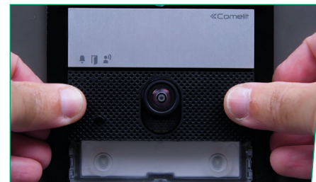
7. ATTACH the audio/video module, button modules and nameplates
