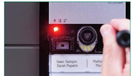
9. THROUGH the dedicated selector, enter the programming mode (you know you are in the programming mode because the dedicated LED comes on) and THROUGH dip switch, select the first address to be assigned to the first button
