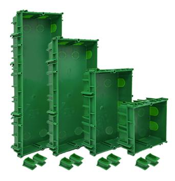
Flush-mounted box for external 1-module entrance panels. Can also be installed in plasterboard walls (using optional accessories). Dimensions (L x H x D):  $123.5 \times 122.5 \times 50$  mm.
