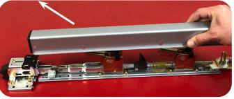
**5.** IF YOUR DEVICE HAS DOGGING, FLIP BASERAIL OVER & REMOVE (2) SCREWS SECURING DOGGING ASSEMBLY TO RAIL. IF YOU HAVE AN OLDER DEVICE WITH RIVETS, YOU WILL NEED TO DRILL THEM OUT OR USE A PIN PUNCH TO KNOW THEM OUT.
