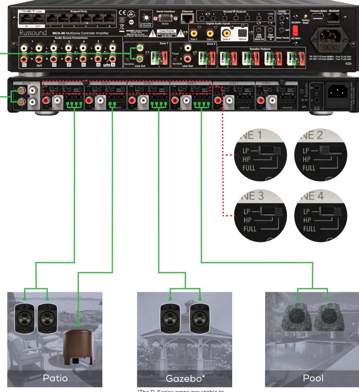
\*The D-Series amps are stable to 4 ohms, so you can add 2 pairs of speakers where needed.
