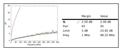
stronger signal. Noise is made up of two parameters – near-end crosstalk (NEXT) and return loss (RL). Putting these parameters together will provide a signal to noise ratio (SNR).
