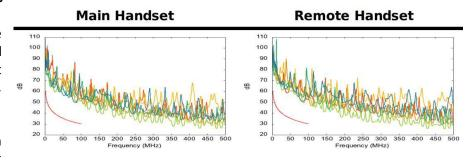
to the limit line, which is of most concern by the contractor and end user. Worst-case value is the amount of margin at the point where the value was the worst overall, but not in relation to the limit line. And because the tester looks for worst-case margin and worst-case value for all pairs and pair combinations, the worst-case margin and worst-case value might not be on the same pair. They can, however, be the same value on the same pair.
