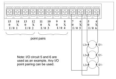
Figure 3.15 Two-Wire Class A Smoke Detector Connections
