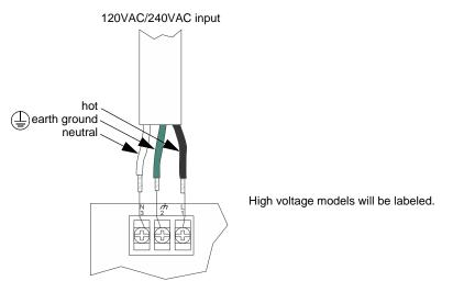
Figure 3.3 AC Power Connection
