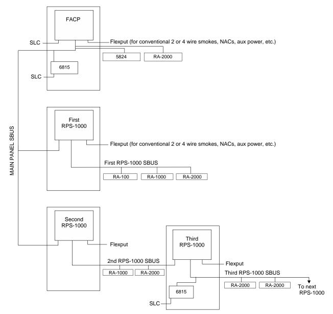
Figure 1.2 RPS-1000 Installation Overview (Details Added)
