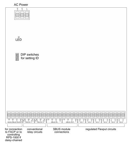
Figure 2.1 RPS-1000 Board Layout
