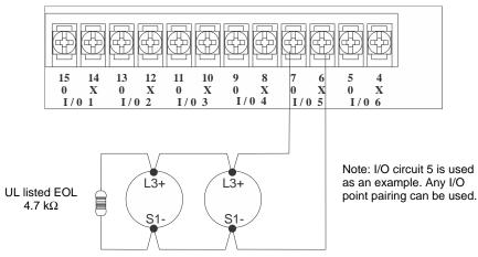
Figure 3.14 Two-Wire Class B Smoke Detector
