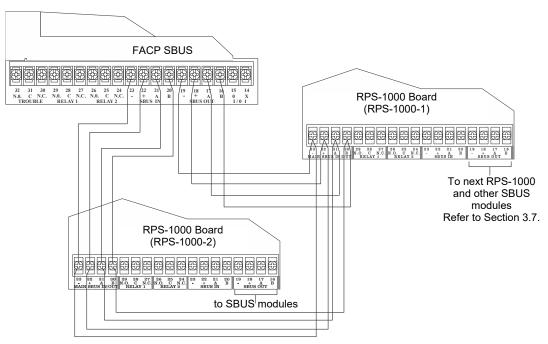
Figure 3.6 Class A RPS-1000 Connection to FACP
