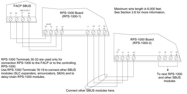
Figure 3.5 Class B RPS-1000 Connection to FACP
