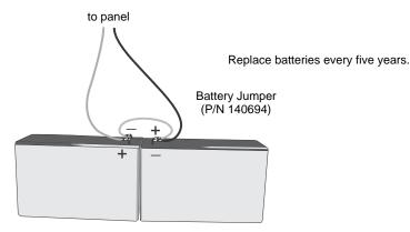
Figure 3.4 Battery Connection
