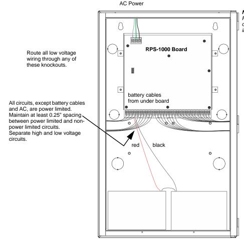
**Note:** Board assembly shown without Formex cover for illustration purposes only. Formex cover must be used in all installations.
