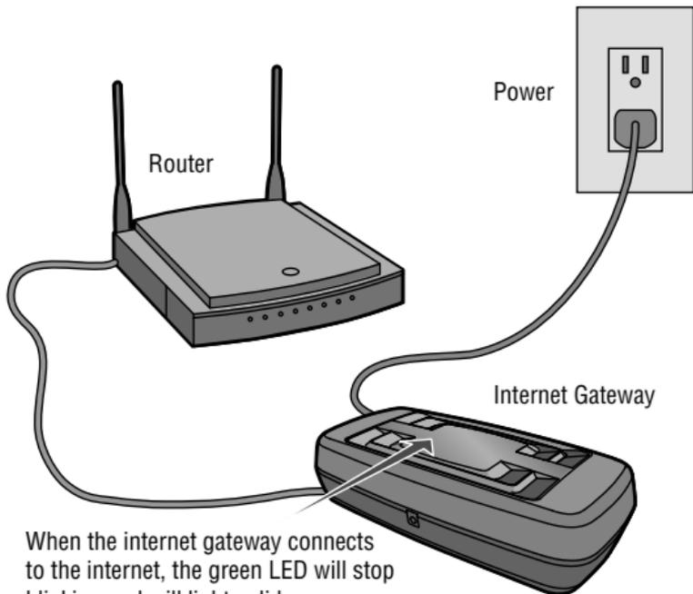
When the internet gateway connects to the internet, the green LED will stop blinking and will light solid.
