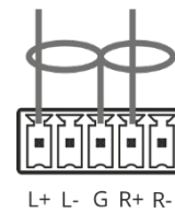
Figure 4: Connecting to an Unbalanced Stereo Audio Acceptor
