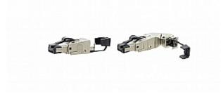
CON-FIELD and CON-FIELD-360 are high-bandwidth, shielded RJ-45 connectors used for terminating Kramer LAN cables. This connector requires no crimping tool to install, and provides fast and reliable termination of shielded twisted-pair cables in the field. The connector is suitable for 10Gb Ethernet (IEEE 802.3an), remote powering (PoE, PoE plus, UPoE) and HDBaseT.
