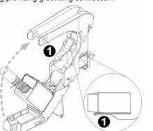
Locate "UP" signs 2 embossed on the locking latch 1 of the jack and the swinging bracket 3. Insert the jack 1 into the opening in the swinging bracket 3 from behind, starting with its lower part, and catch the edge of the opening between two tabs on the bottom part of the jack. Push the jack firmly until it snaps securely in the opening. The jack's latch shall snap behind the upper edge of the opening.
