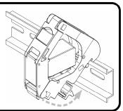
Place side lids 1 where necessary. When using DIN-rail mounting modules in series, side lids may be installed on end modules only.
