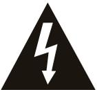
The lighting flash with arrowhead symbol, within an equilateral triangle, is intended to alert the user to the presence of uninsulated “dangerous voltage” within the product’s enclosure that may be of sufficient magnitude to constitute a risk of electric shock to persons.
