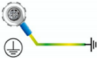
Figure 1: Socket-outlet protective earthing connection
