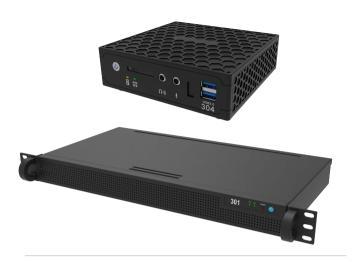
The Wisenet SKY Bridge acts as a gateway from your premises to the Cloud Data Center where your video is stored and managed. The bridge provides video buffering, a secure connection, bandwidth management, and monitoring of cameras.
