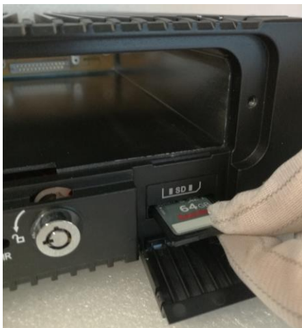
Figure 1. 15 Insert SD Card
