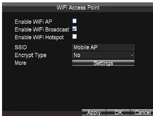
Figure 7. 5 Wi-Fi Access Point Settings
