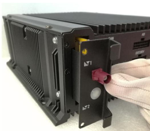
Figure 1. 19 Plug the SIM Card
