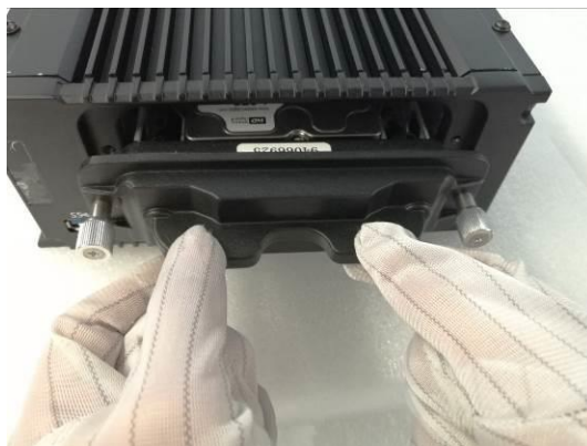
Figure 1. 14 Pull Out Hard Disk Box
