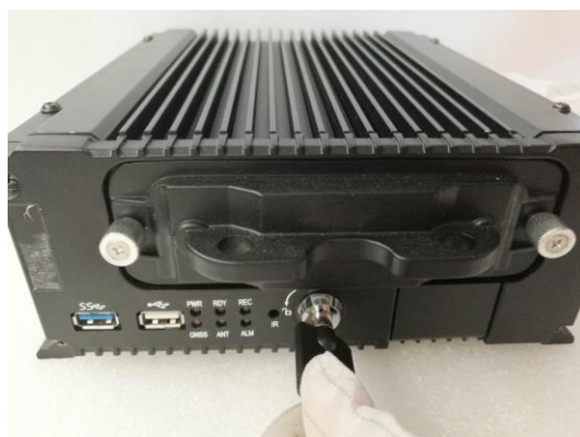
Figure 1. 9 Lock Hard Disk Lock
