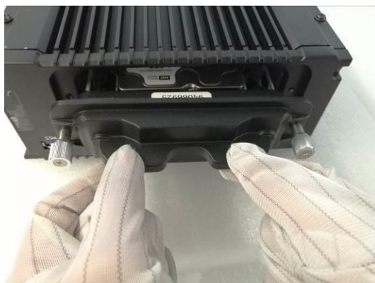
Figure 1. 10 Pull Out Hard Disk Box
