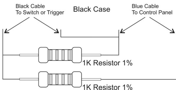
Normal Resistance: 2K  $\Omega$ ; Alarm Resistance: 1K  $\Omega$
