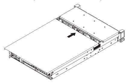
$oldsymbol{8}$  Secure the cover using the screws that had been removed at step 2.
