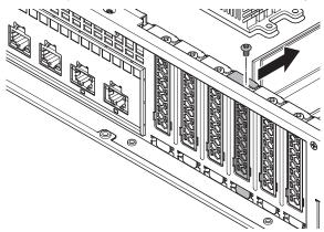
Insert the SSD card into the slot.
