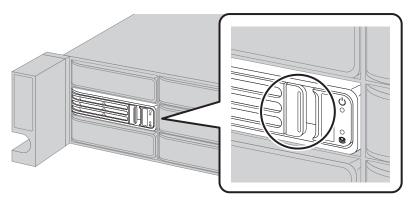
$\boldsymbol{3}$  Pull out the drive cartridge and remove it from the TeraStation.
