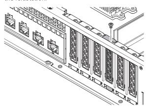
**7** Return the rear top cover back and slide it into the secure position.
