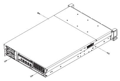
**3** Slide the rear top cover to the back side and lift it up to remove it from the TeraStation.
