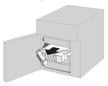
$\boldsymbol{5}$  Insert the new drive into the empty slot with the lock mechanism remaining open.
