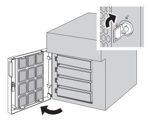
$\boldsymbol{2}$  Remove the front cover while holding the hook downward.
