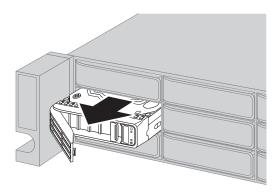
**4** Insert the new drive into the empty slot with the lock mechanism remaining open.
