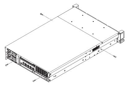
Slide the rear top cover to the back side and lift it up to remove it from the TeraStation.
