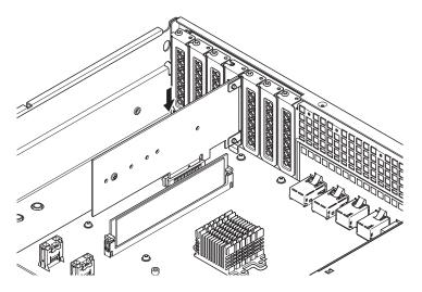
**6** Secure the card using the screw that had been removed at step 4.
