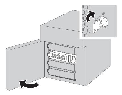
$oldsymbol{3}$  The failed drive's status LED will be glowing red. Push its unlock button and swing the lock mechanism out.
