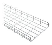
The construction of the nVent CADDY WBT Performance Cable Shaped Wire Tray eliminates stress and pressure points on today's high-speed/performance cabling media. The backbone of the platform features our "Shaped Tray" technology—offering substantial support improvement over traditional wire mesh tray. This technology increases support by 400% while reducing cable strain up to 65%, protecting high performance and fiber optic cable for the life of the installation.
