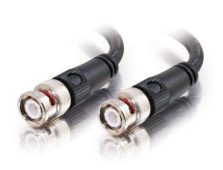
A high quality BNC cable for video applications including CCTV, broadcast, studio, boardroom presentations, home theater, etc. Manufactured from 75 Ohm RG59/U dual shield coax cable (60% copper braid over foil) with a 22 AWG copper-covered steel center conductor. Finished with bright nickel-plated BNC connectors that have molded PVC strain relief to protect the cable from wear over time.
