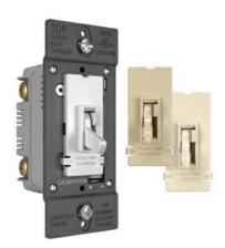
TradeMaster® Toggle Slide Dimmer is designed for use with compact fuorescent or LED lighting fixtures. This single pole 3-way switch can be used in a two-location layout. The slide can be set to your preferred level and then toggle on and off providing instant repeatablility.
