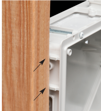
Positioning tabs are set for 1/2" or 5/8" drywall.
