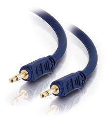
This cable is specifically designed to provide quality signal transfer for mono audio and data transfer applications. It features two 27 AWG oxygen-free copper conductors, a drain wire, an aluminum foil shield to prevent unwanted EMI/RFI interference, and fully molded, gold-plated connectors providing strain relief for a quality connection.
